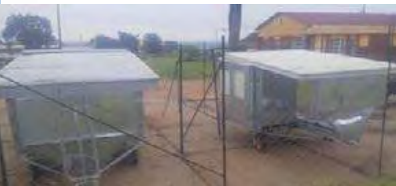
The two Night-Day solar crop drying and Water Recovery machines assembled side by side in the Engineering Faculty compound (Left: 150 kg capacity; Right: 200 kg capacity)
