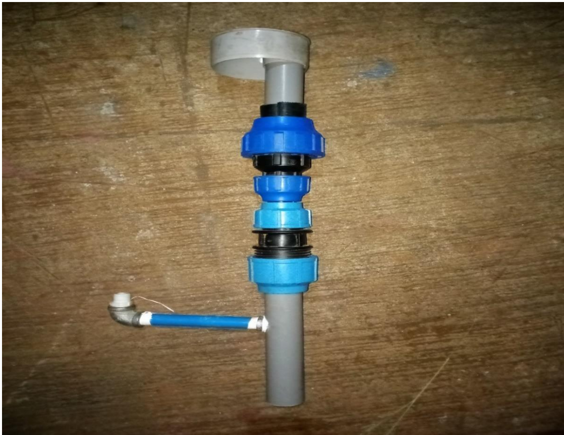
Figure 7 showing the venturi tube
