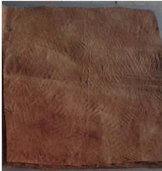
FIG. 1. Bark cloth non-woven laminar fabrics. [Color figure can be viewed in the online issue, which is available at wileyonlinelibrary.com .]
